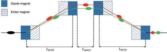
FIG. 3. The schematic of dipole-kicker combination in a typical 4-rectangular-dipole chicane.
