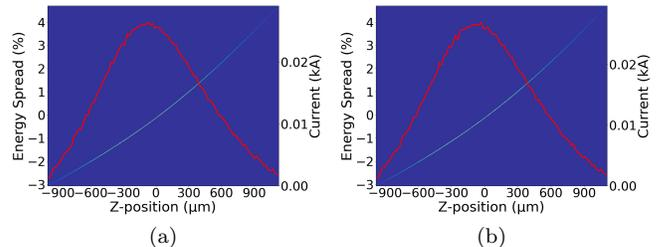
FIG. 7. Longitudinal phase space distributions at the BC1 end of two modes. (a) for mode 1, (b) for mode 2.
