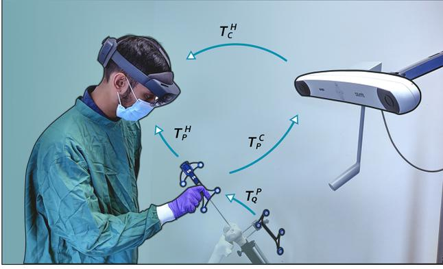
Fig. 3. Various transformation matrices generated when using system: tool pose in fixed virtual world frame,  $T_P^H$ , tool pose with respect to surgical robot's optical tracker,  $T_P^C$ , and calibration matrix which maps between optical tracker and virtual coordinates,  $T_C^H$ .  $T_Q^P$ , matrix describing relative pose between two IR marker-arrays.
